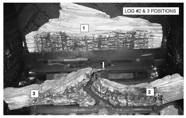
5. Identify the 1/4" Pins located on the top surface of the Rear Burner and on the top surface of Log #2.
